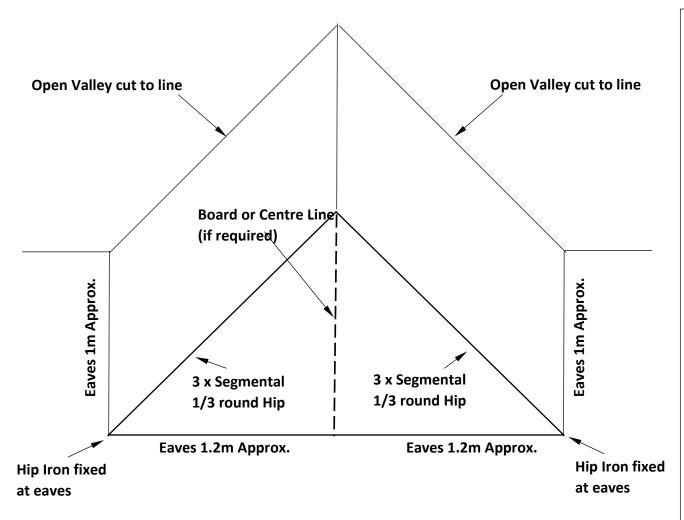
The drawing shown is typical of hip to valley model roofs used in colleges and training centres in the UK. It is envisaged that existing rigs will be adequate without the need for new rigs or significant adaption. Any queries relating to the rigs should be discussed with the CITB Judge before the heat takes place.
