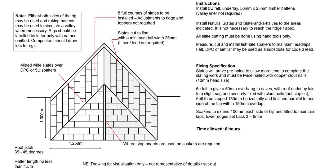
NB: Centres should use stop boards, valley battens, lines etc to keep within these dimensions to ensure consistency across the heats. Where this is not possible, any adjustments should be agreed with the SkillBuild appointed judge and/or NFRC before the heat is confirmed
